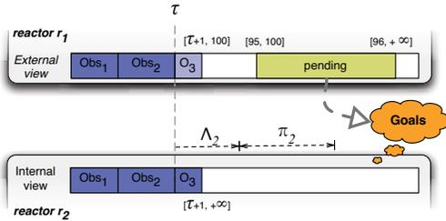
Figure 6: Transfer of a pending token to its corresponding goal set. Reactor  $r_1$  has a pending token overlapping the planning window of  $r_2$  to be inserted in its goal set.
