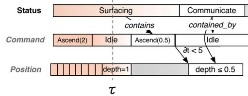
Figure 7: A partial plan produced by the *Pilot* after an initial plan failure based on Fig. 3. Red areas before  $\tau$  indicate past observations grounded by synchronization.
