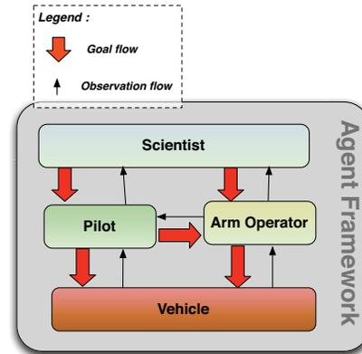
**Figure 2:** An agent is composed of multiple reactors or control loops.
