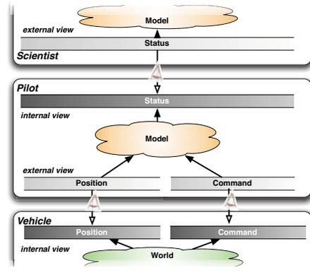
Figure 5: Relationship between internal and external views of a state variable. The internal view is deduced based on the reactor's model; the external view "observes" the state variables owned by a different reactor.
