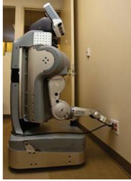
Figure 8: *PR2* plugging in to a standard outlet.
