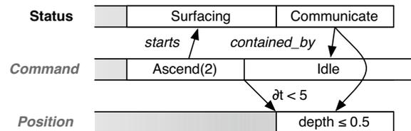
**Figure 3:** The *Pilot's* plan for communication: *Status* is *internal* while *Command* and *Position* are *external* to this reactor.
