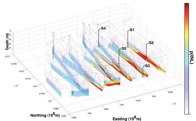
Figure 10: Visualization of a survey mission to detect and characterize a dynamic ocean feature. High probability of feature presence is indicated in red. S1-S5 indicate triggering of 10 water samplers.
